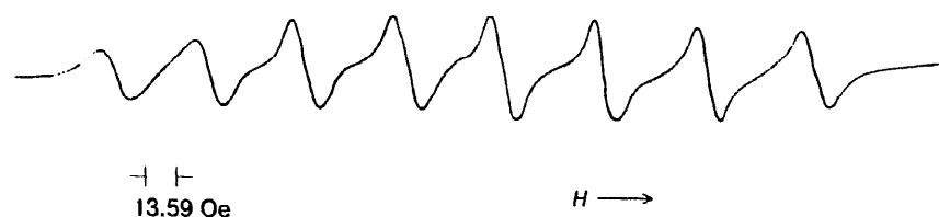
Fig. 2. ESR spectrum of anion-radical obtained in electrochemical reduction of XVIII at E_{\text{gen}} = -1.30 V, Pt electrode in MeCN, 0.1 M \text{Et}_4\text{NBF}_4 related to Ag, c = 10^{-3} mol/l at 293 K.
